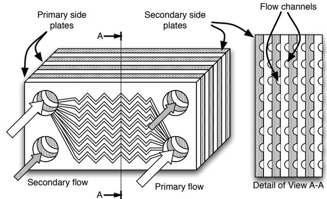
Figure 1. EXAMPLE OF COMPACT HEAT EXCHANGER CORE SHOWING LAYERED PLATES AND MICRO-CHANNELS
