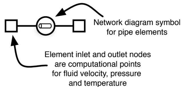
Figure 10. PIPE ELEMENTS CREATED FOR CHANNEL NETWORK
