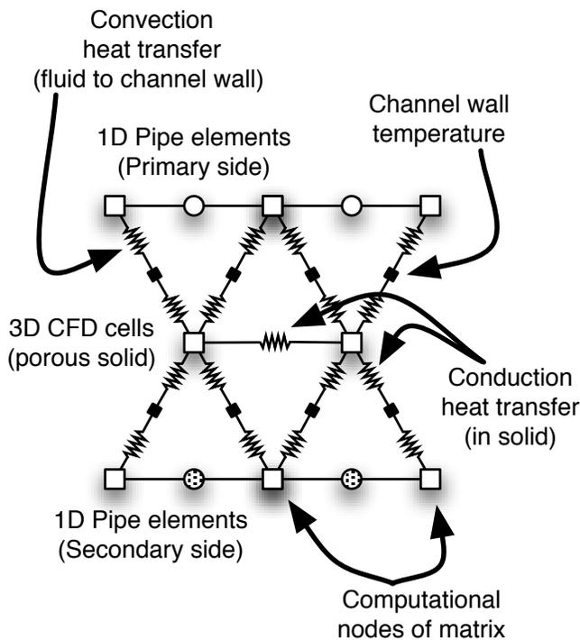
Figure 11. CONNECTIVITY BETWEEN THE 1D PIPE ELEMENTS AND THE 3D CFD CELLS IN THE HEAT EXCHANGER CORE
