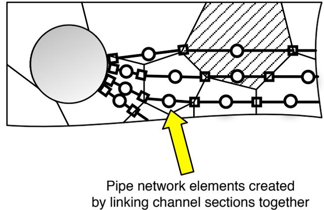
Figure 9. DETAIL OF CFD MESH WITH TRACED CHANNELS SUPERIMPOSED ON THE GRID
