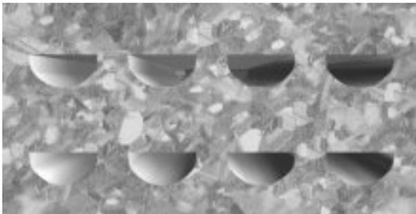
Figure 5. DIFFUSION BONDING PROMOTES GRAIN GROWTH BETWEEN PLATES FOR IMPROVED HEAT EXCHANGE [3].
