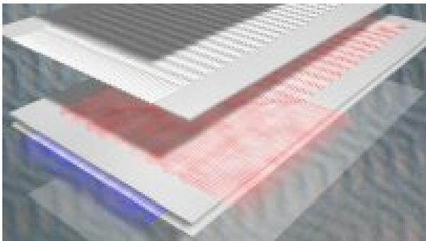
Figure 4. DIFFERENT PLATE LAYERS ARE STACKED UPON EACH OTHER TO FORM PRIMARY AND SECONDARY SIDES [3].
