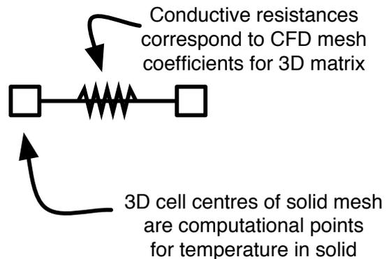
Figure 8. HEAT FLUX BETWEEN 3D CELLS IN EXCHANGER CORE
