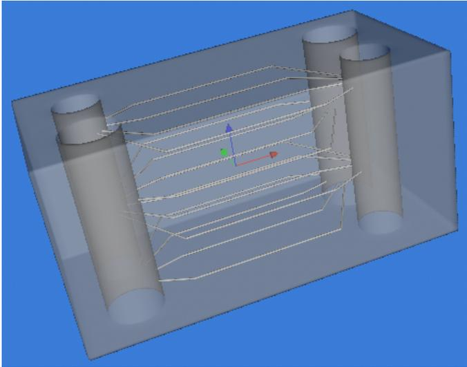
Figure 6. DEMONSTRATION HEAT EXCHANGER GEOMETRY
