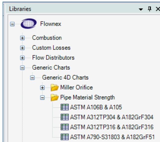
Figure 3: Piping and Flange Material Strength Library
