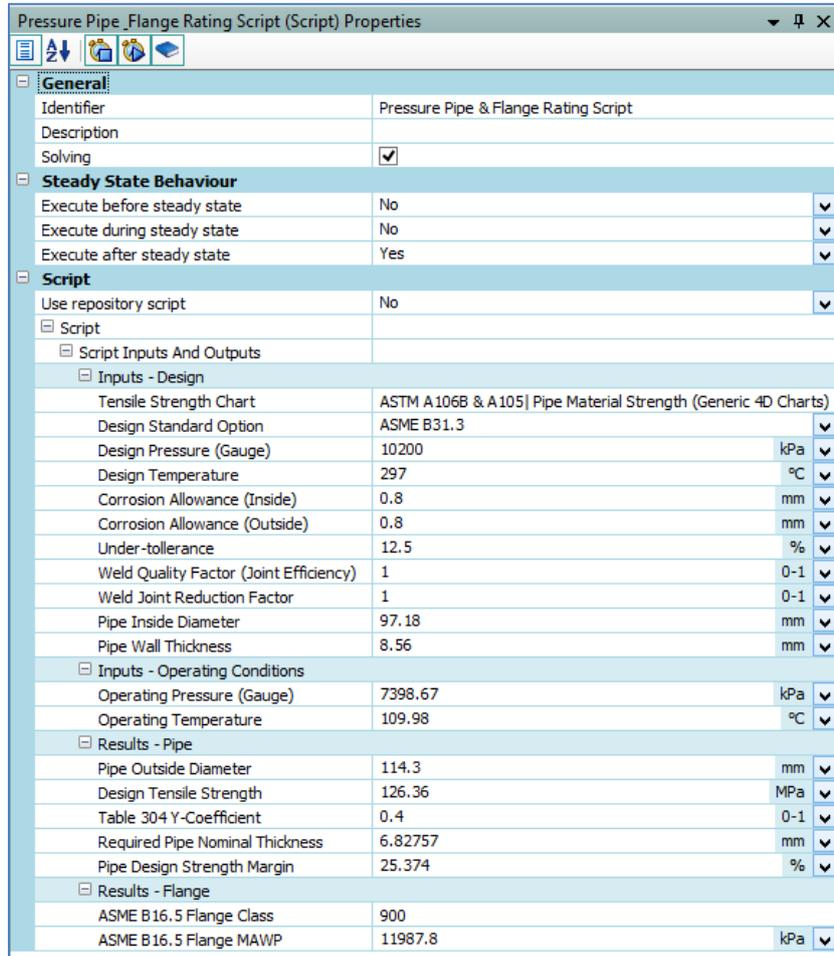
Figure 2: Pressure Piping and Flange Rating Calculation Script Inputs and Results
