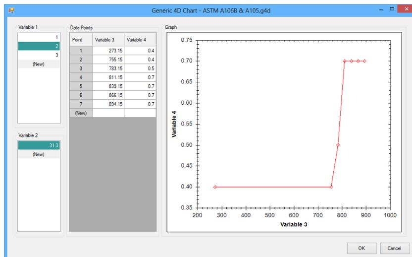
Figure 5: ASME B31.3 Y-Coefficient from Table 304.1.1
