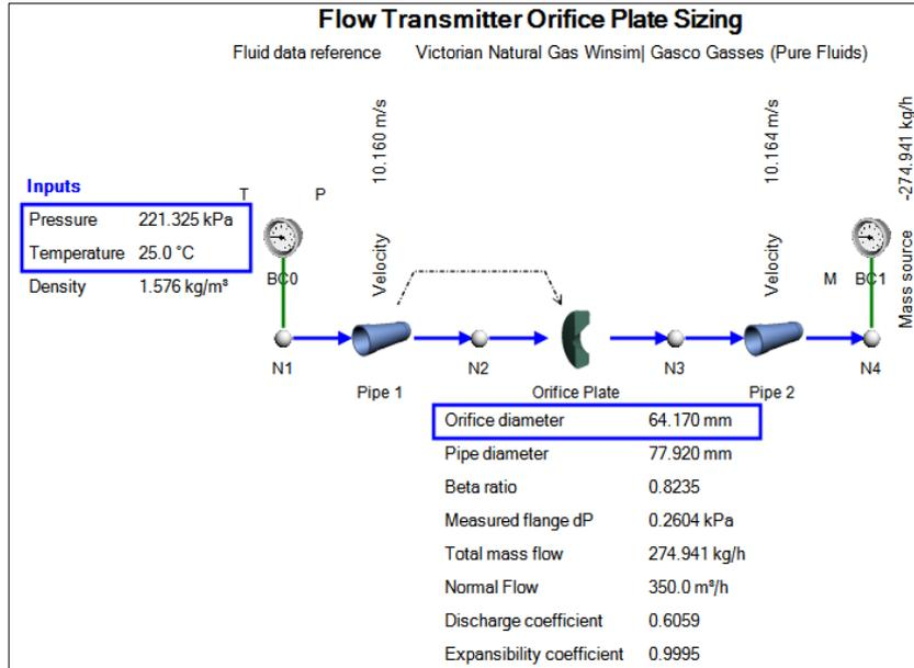
Figure 5: Testing the Low Flow Case (0.3 kPa measured).
