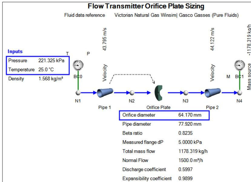
Figure 1: Example Flownex Orifice Plate Pipe Network.
