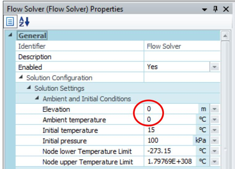
Figure 3: Ambient Conditions: 0°C at 0 m Elevation (101.325 kPa).
