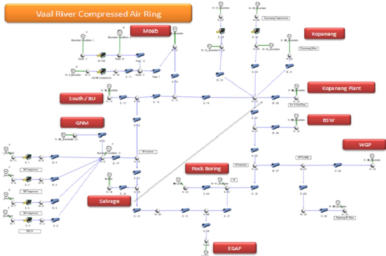
Figure 1: Flownex simulation of the compressed air network.
