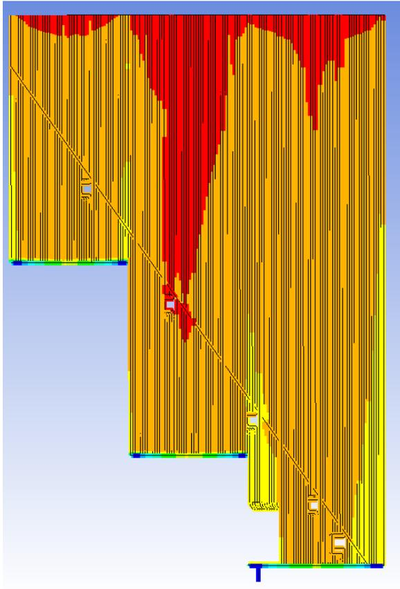
Figure 7: Solved thermal field in Flownex (Front Wall)
