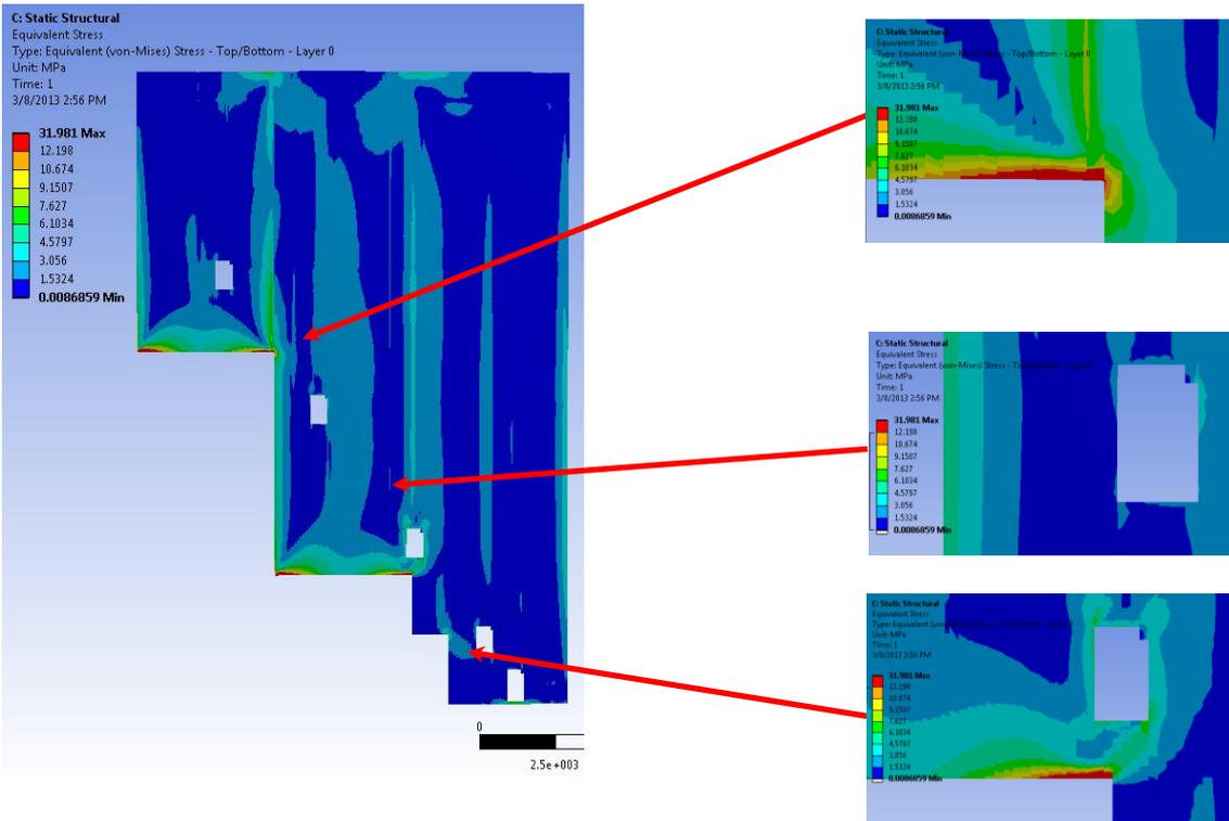
Figure 8: Thermal Stress Results (Tube wall only)
