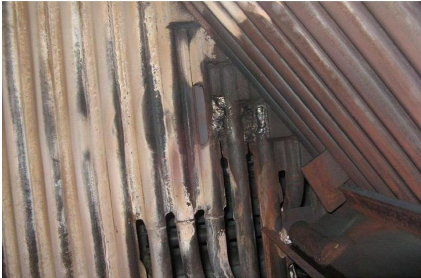
Figure 1: An example of typical boiler tube failure locations
