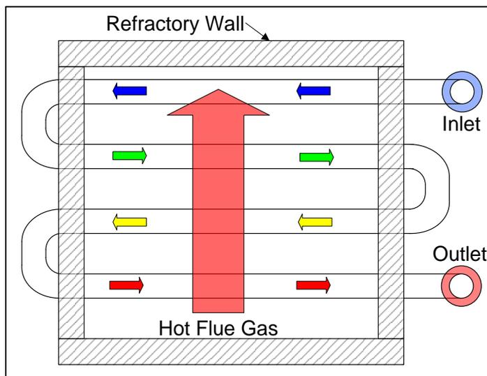
Figure 1: Simplified layout of the fired heater.
