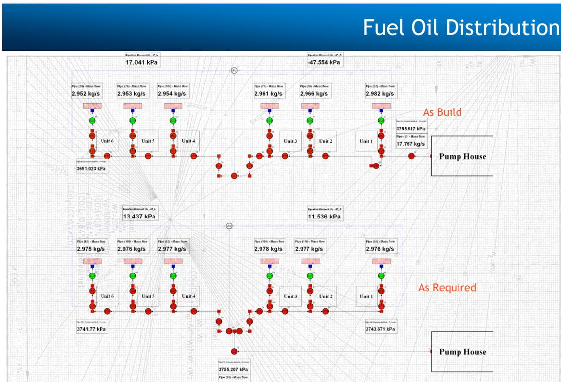
Steinmüller can calculate the system resistance and associated pressure drop with the fuel oil distribution pump at different positions. This provided Steinmüller with the pressure difference over the system and determined the impact of the different layouts on the fuel oil distribution pump.
