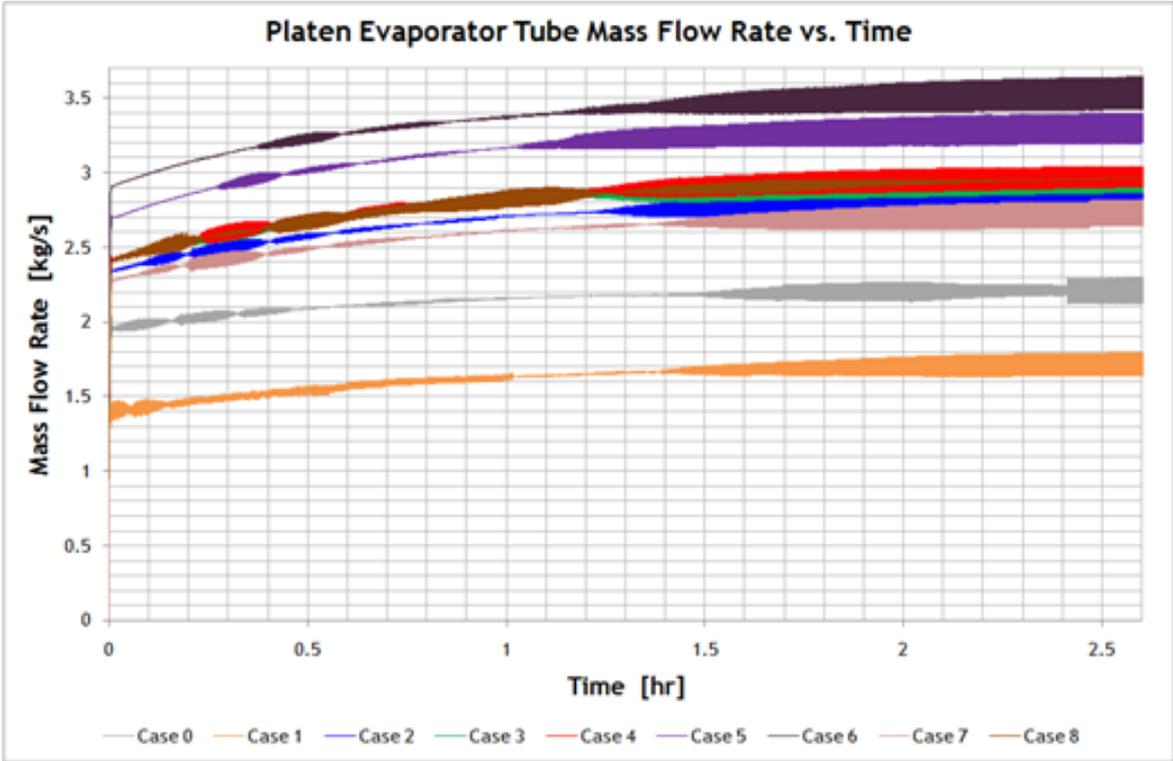
Figure 3: Tube Mass Flow distribution for Case 0 - 8.
