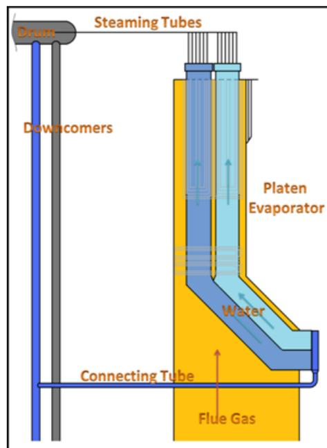
Figure 1: Schematic representation of the simulation model.
