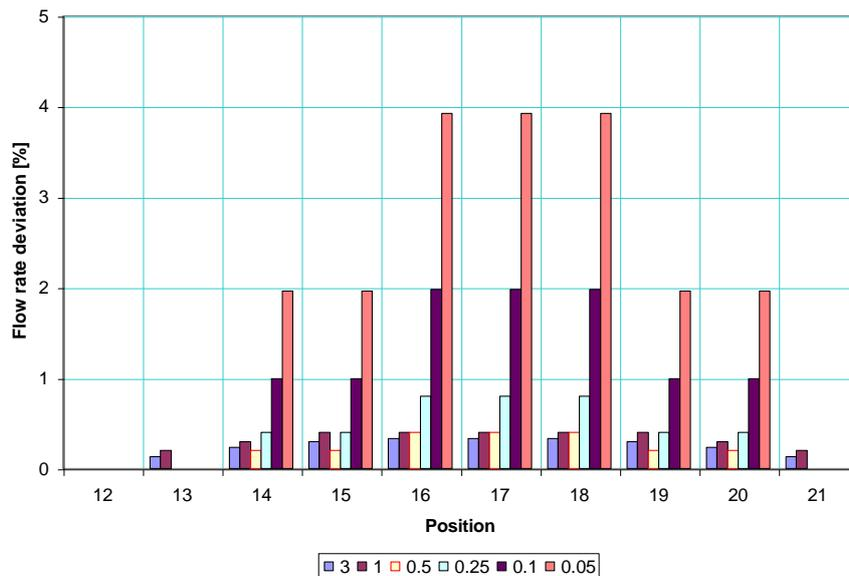
Figure 4: Simulated deviation in flow rate at the different openings for various different total flow rates.
