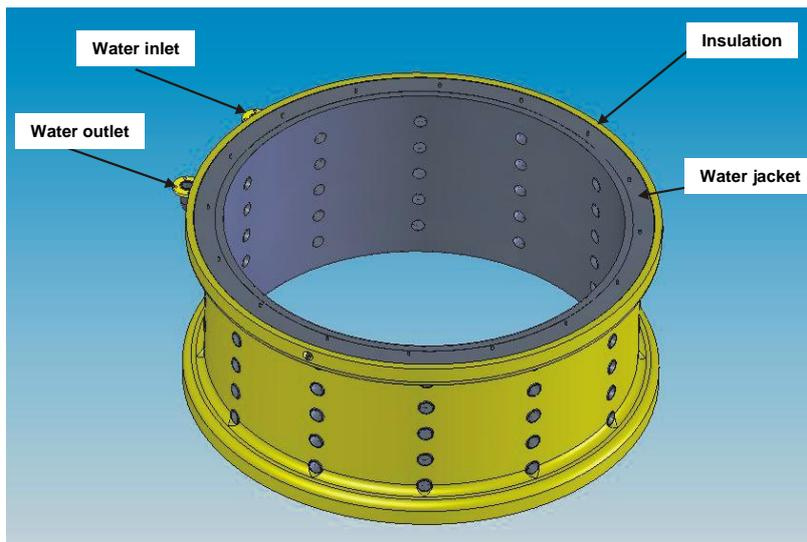
Figure 1: Solid model of the water jacket layout.
