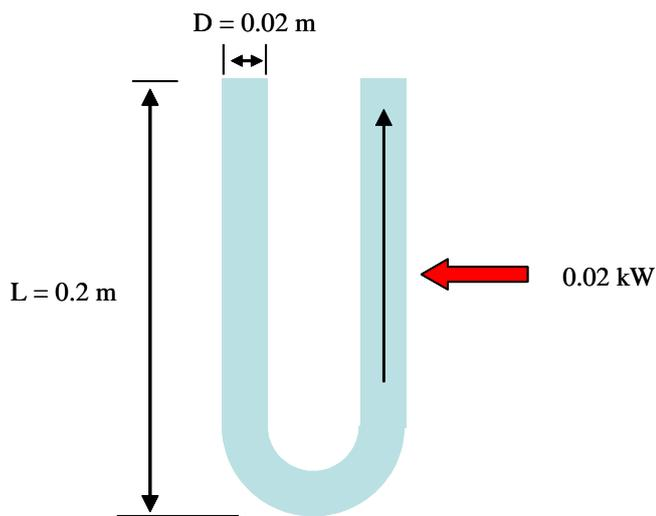
Figure 1: Schematic layout of a U-tube in which air is flowing due to natural convection.
