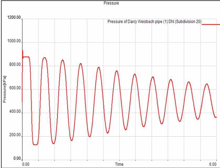
Figure 3: Water hammer simulation results.
