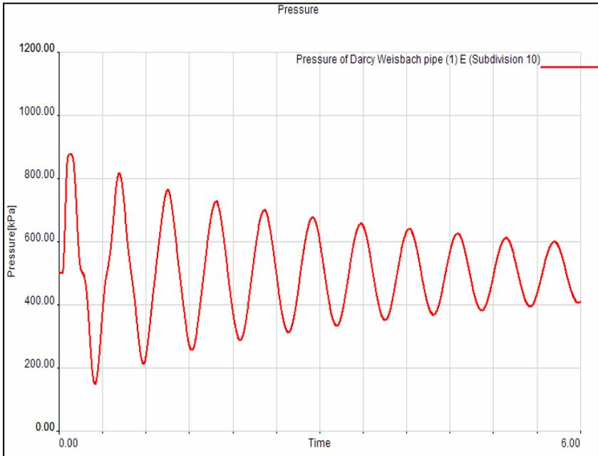
Figure 4: Water hammer simulation results.
