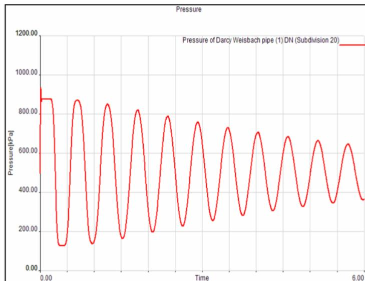
Flownex takes the elasticity of the fluid and pipe wall into account
