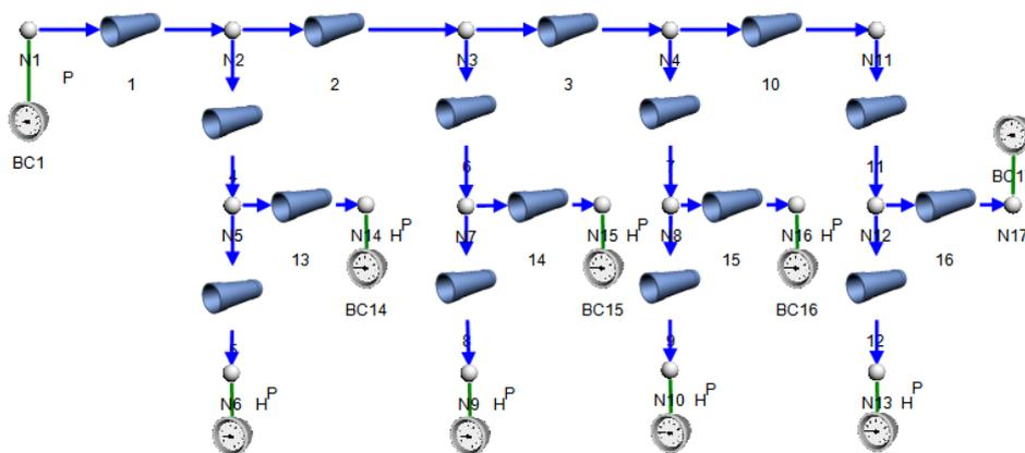
Flownex was used to calculate the flow and temperature distribution in a chilled water reticulation network for a deep mine.
