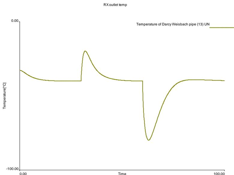
Figure 3: Temperature at the outlet of the recuperator primary side.
