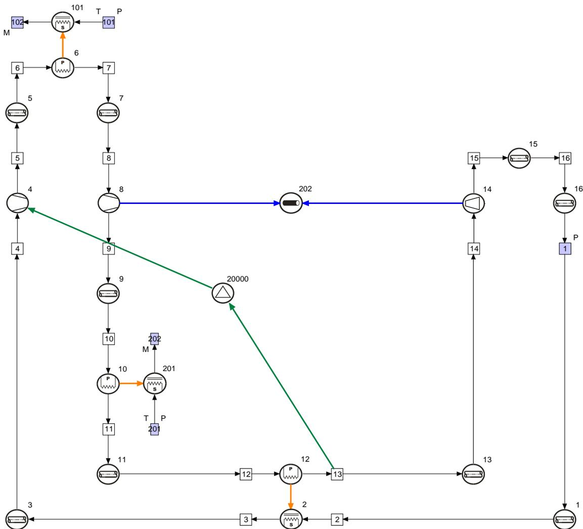
Figure 1: Flownex network of the direct two-shaft closed inter-cooled recuperated Brayton cycle PBMR power plant.
