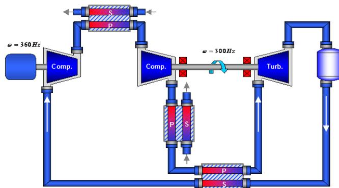
The transient simulation of the two-stage air cycle chiller integrated with the PID controller shows that the temperature can be controlled effectively by varying the shaft speed of the low pressure compressor.
