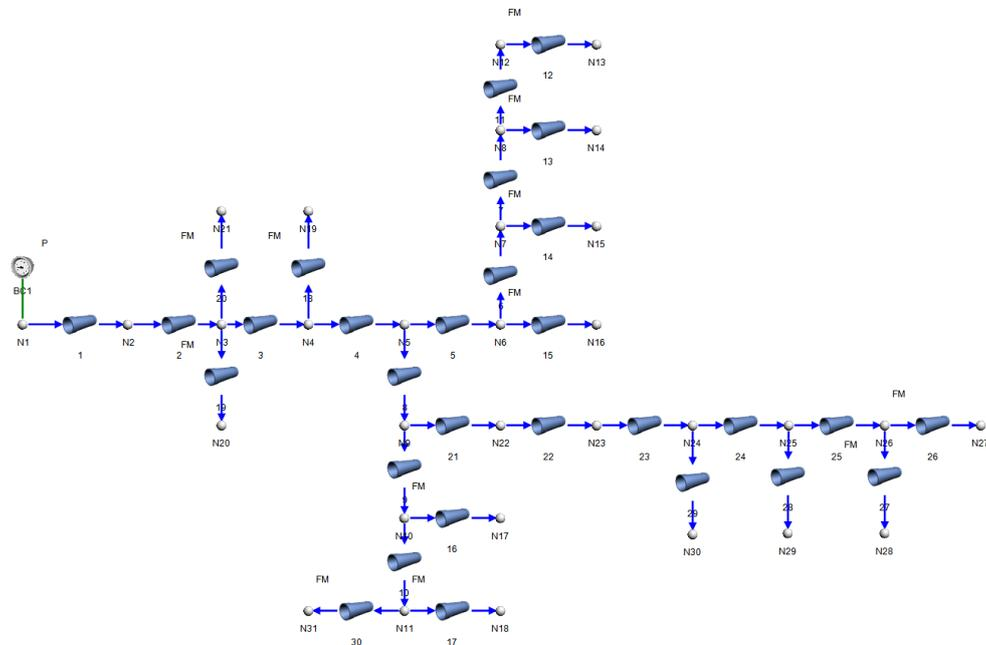
Flownex has a built in orifice sizing capability specifically designed to assist in modeling flow balancing problems.
