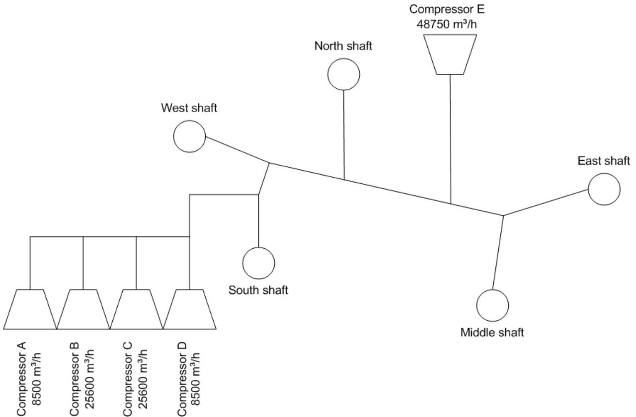
Figure 1: Schematic layout of the compressed air network.
