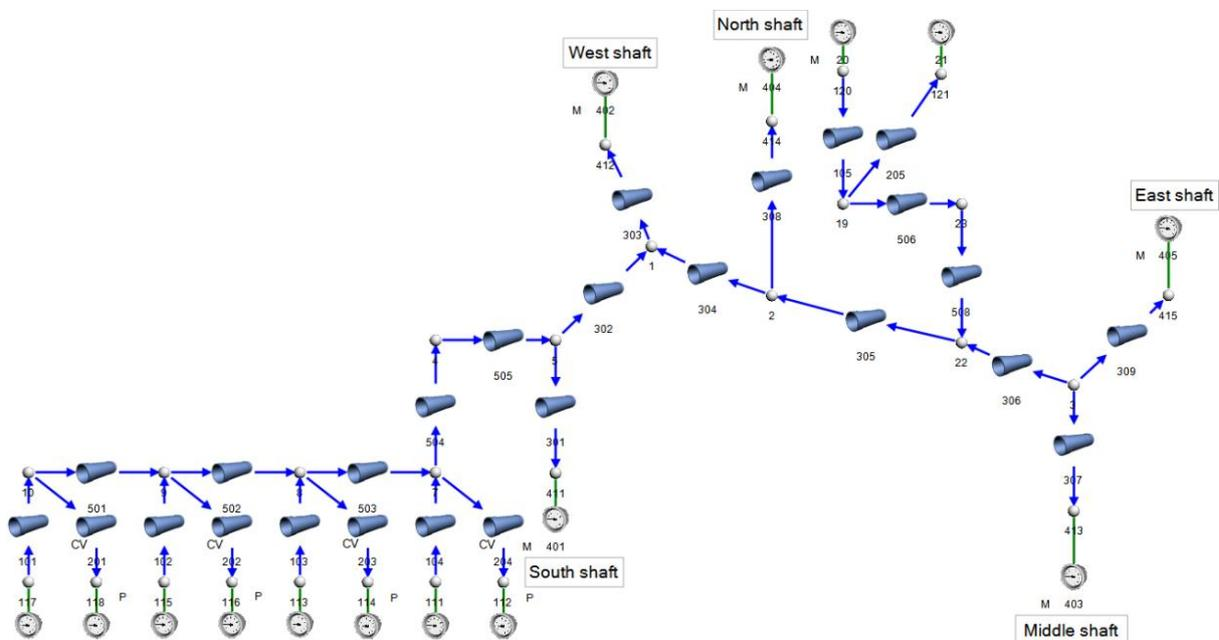
The Flownex simulation will verify whether the compressed air network can maintain the required minimum shaft pressures when the production figures increase in the future expansion of the mining activities.
