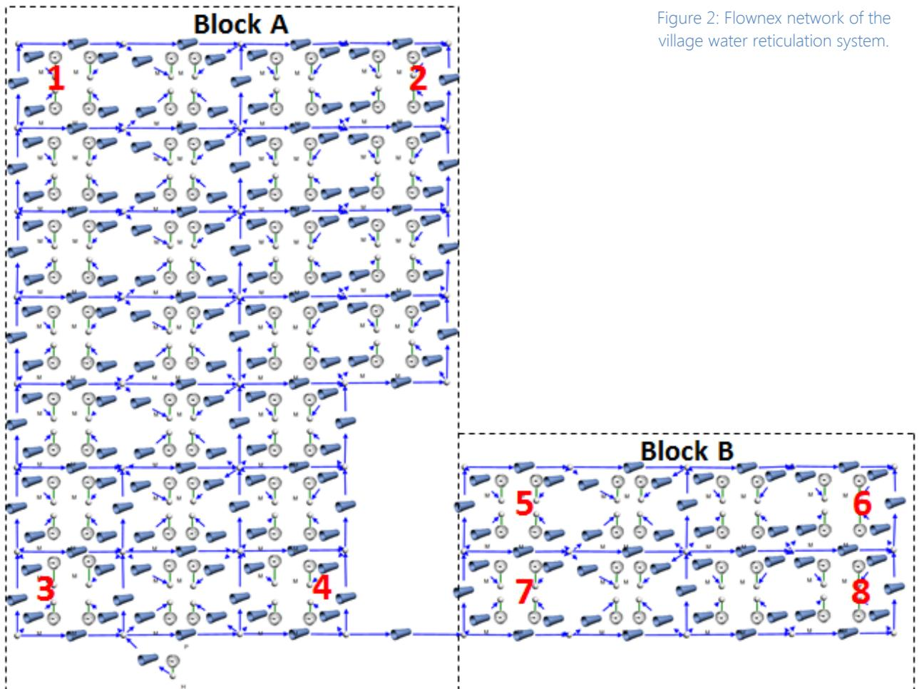
Figure 2: Flownex network of the village water reticulation system.
