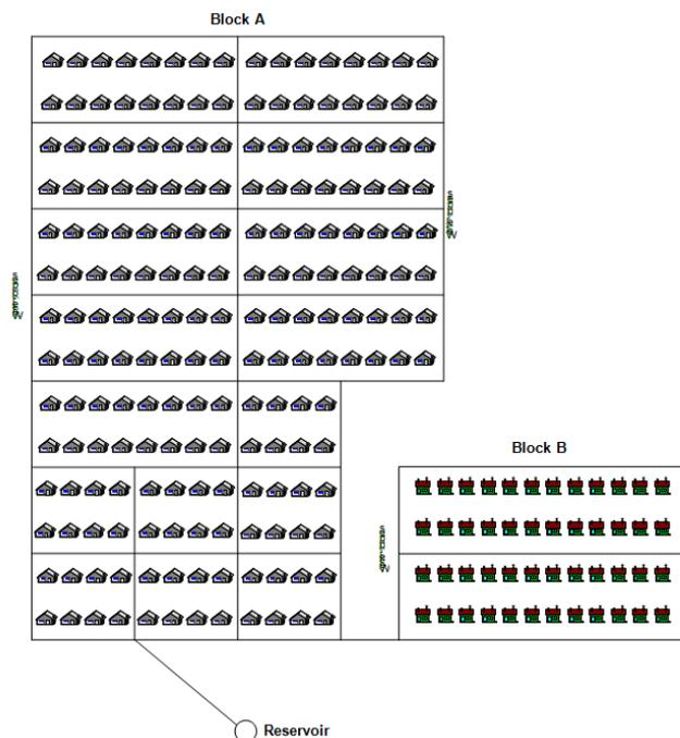
The optimization and design capabilities of Flownex were used to optimize the system and maintain adequate water pressures during peak demand.
